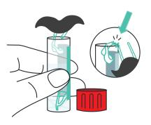
Do this by bending the swab arm against the edge of the tube at the break line.
